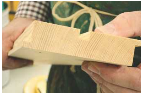
▲ Pic.2 The cross sections of the pulley stiles and head of the frame are identical
